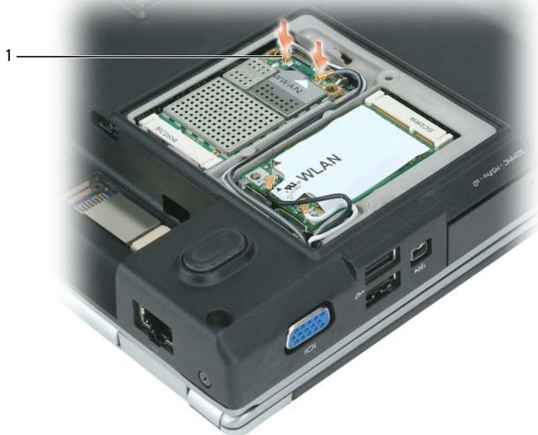
1 Antennenkabelanschlüsse (2)
